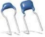
**Important: If your kit includes TANTALUM capacitors for C2-C5, they ARE POLARIZED, and polarity is CRITICAL. If your kit includes MLCC capacitors for C2-C5 they are not polarized and the polarity markings on the circuit board may be ignored.**
