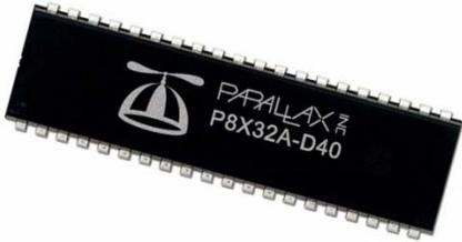
As with ALL ICs, it's POLARIZED. Insert into the PC board with the Pin 1 end (indicated by a notch on the short side, on the left as shown in this illustration) facing to the LEFT (this is the only IC that faces LEFT).
