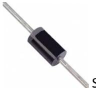
Similar in appearance to D1 but “fatter” and with thicker leads. POLARIZED. Must be installed with banded end down matching circuit board silkscreen.
