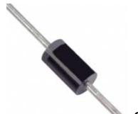
Similar in appearance to D1 but “fatter” and with thicker leads. POLARIZED. Must be installed with banded end down matching circuit board silkscreen.
