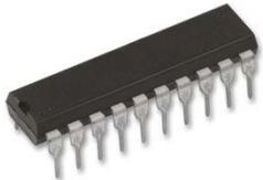
POLARIZED. The notched end, pin 1, faces right when installed in the sockets.
