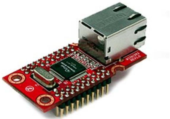
Polarized, must be plugged in with LAN connector facing left.
