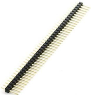
This may be supplied as a single long header that must be snapped to the needed lengths or cut with diagonal cutters, or may be supplied as 7 individual parts. What's needed are five 3-pin headers, one 4-pin header, and one 2-pin header. The short legs of the headers are inserted into the circuit board, the long legs are where the shunts (jumpers) are plugged. Not polarized.
