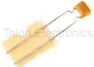
Appearance is similar to the tantalum capacitors but these will generally be smaller. There will be 7 or 9 identical capacitors depending on board date code. Not polarized. Lead lengths are the same.
