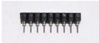
Note: a 9-pin SIP socket is shown, 2 32-pin SIP sockets are supplied. Not polarized.
